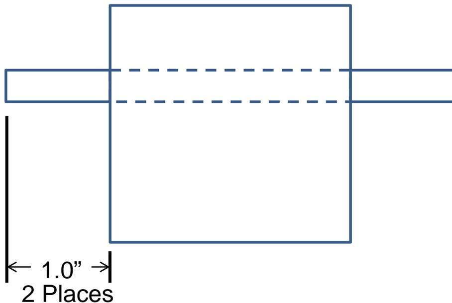
Cut (4) blocks 1.5" x 1.5". Drill and install 5/16" dowels as shown above.
